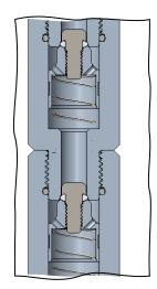
The 20,000 psi rated KRATOS ¼" check valve is configurable in series. This is possible by utilizing the "stacking feature" exclusive to the KRATOS check valve with the series adapter.
